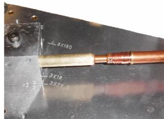
13. Once the conductor tube has been properly aligned, remove the tube from the RAT by loosening the index screw #3a.
