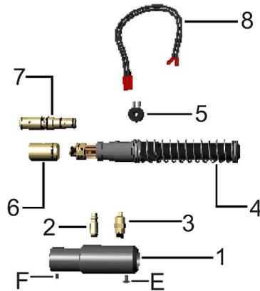
8. With the conduit liner removed from the rear connector plug (#7), Loosen and back the connector plug set screw (F) out to be flush with the O.D. of the plastic rear case (#1).
